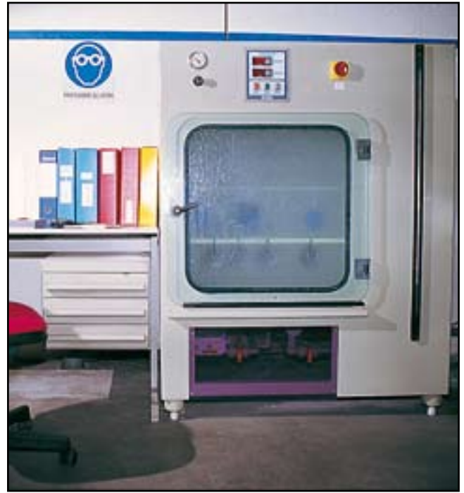
TESTS IN NEBBIA SALINA SALTY FOG TESTS SALZNEBEL TEST TESTS EN ATMOSPHERE SALINE
